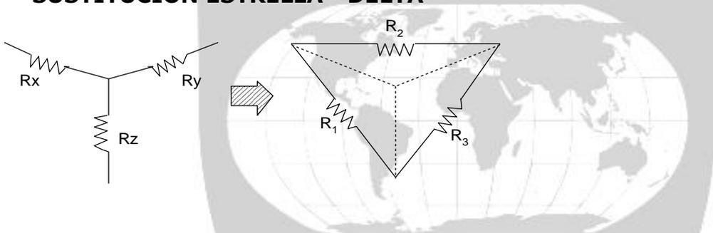
$$R_1 = \frac{R_x R_y + R_x R_z + R_y R_z}{R_y}$$
